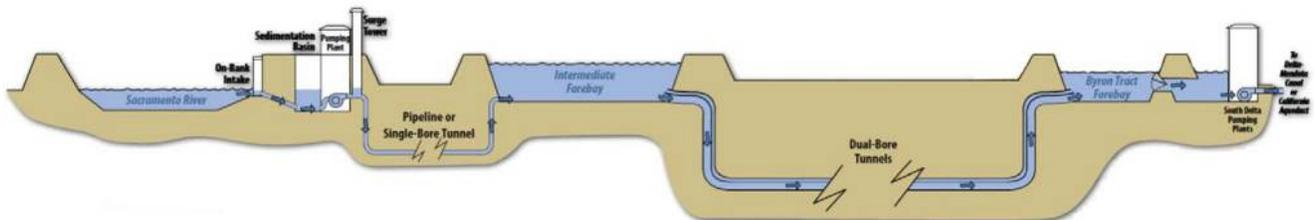
Diagram of proposed Delta pipelines. COURTESY OF THE CALIFORNIA DEPARTMENT OF WATER RESOURCES.
